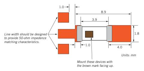
Figure 10 shows the recommended chip antenna layout.
