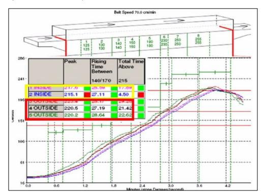
Figure 15. Solder Reflow Curve
