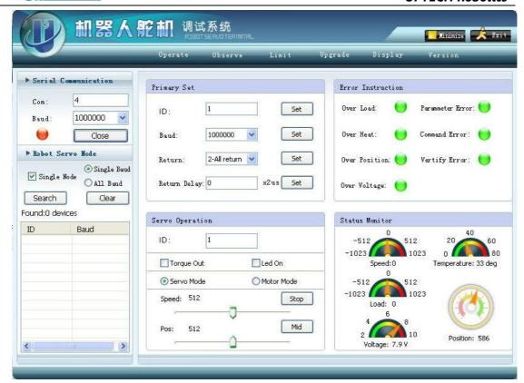
The default baud rate of CDS55xx servo is 1Mbps (1,000,000). User can change baud rate in "Primary Set" window.
