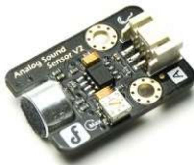
Analog Sound Sensor is typically used in detecting the loudness in ambient, the Arduino can collect its output signal by imitating the input interface. You may use it to make some funny interactive works such as a voice operated switch.
