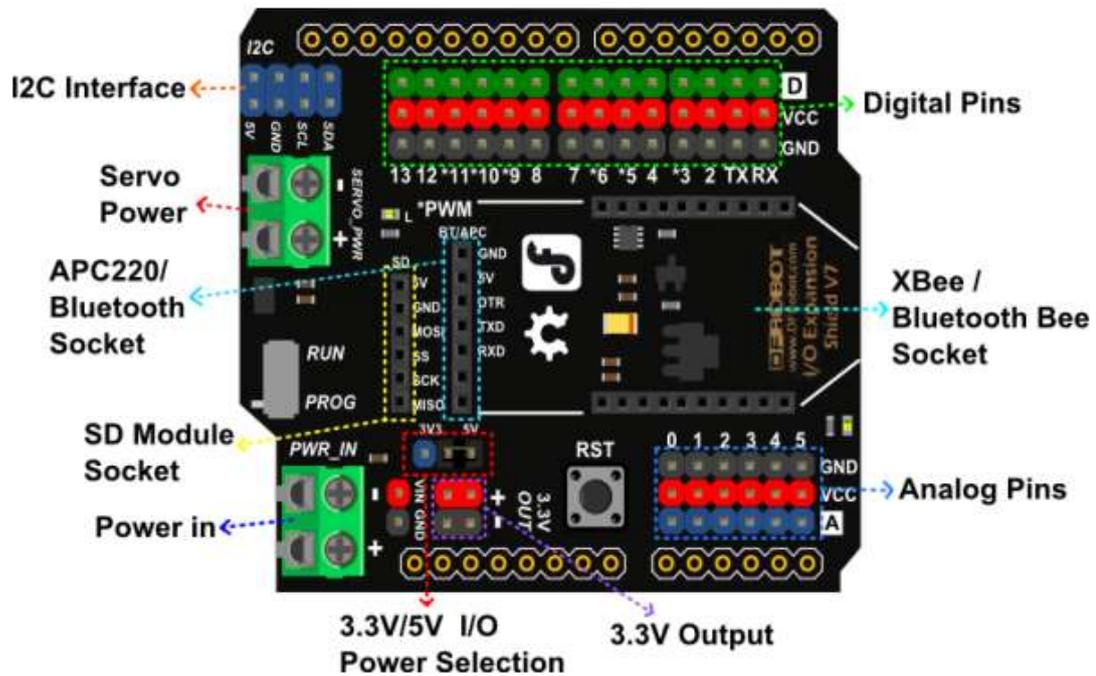
This expansion shield for Arduino will help you to connect your comments to Bluno well, and if you have some other control board such as UNO or Mega2560 or Romeo you can also use this expansion shield. In this kit, it will help you to connect the LED strip and sound sensor. And for more details of V7, click the website below.
