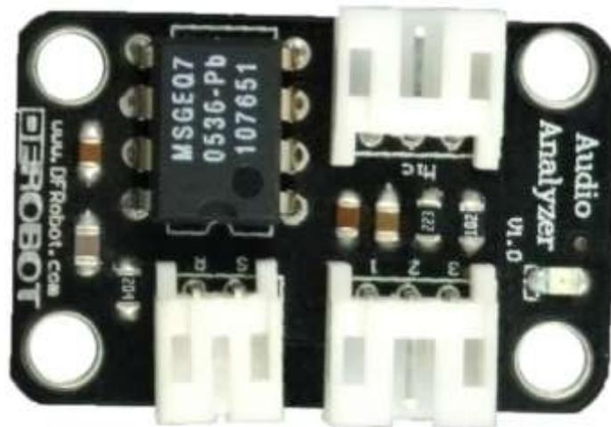
This module features the MSGEQ7 graphic equalizer display filter. It will give your Arduino ears. Sound is broken down into seven frequency bands and the peak level for each band can be read. The seven frequencies measured are as follows: 63Hz, 160Hz, 400Hz, 1kHz, 2.5kHz, 6.25kHz and 16kHz. This module can be used to create sound visualizers, detect patterns in music or add sound activation to your microcontroller.
