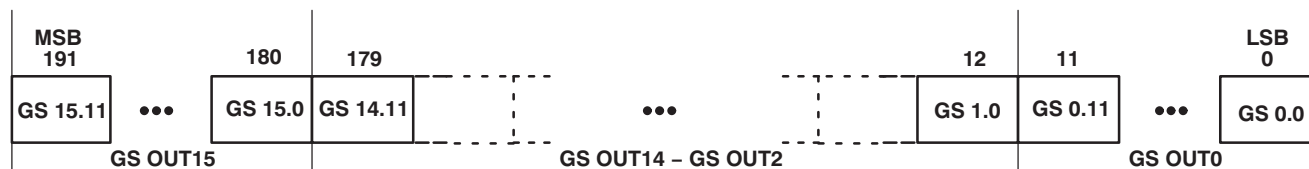
Figure 18. Grayscale Data Packet Format
